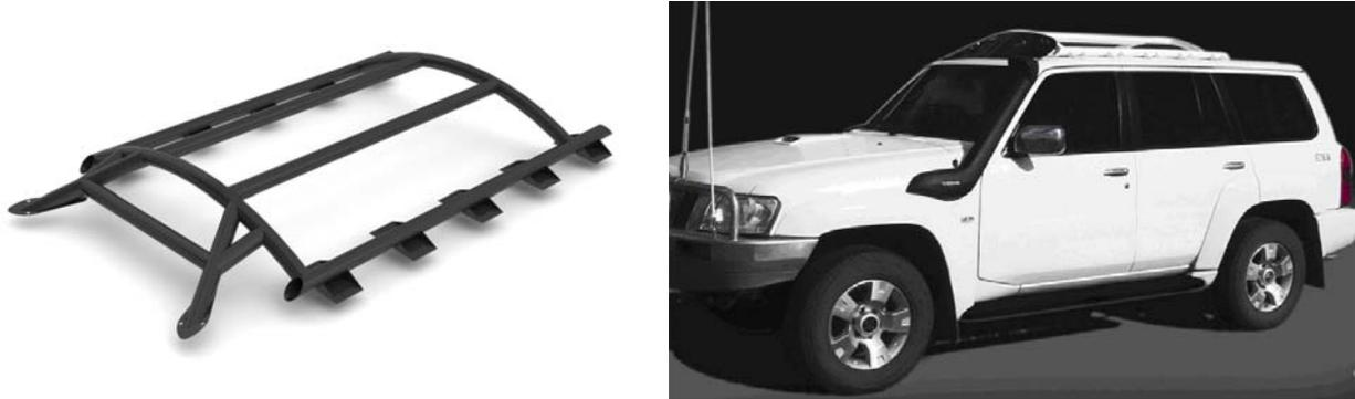
Fig. 5: HALO™ device unattached (L), and affixed to a Nissan Patrol vehicle (R). Note that this vehicle is equipped with a black engine snorkel on the left side.
