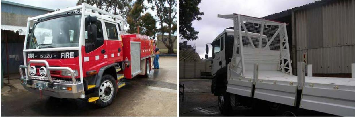
Fig. 4: Two external rollover-protection roof retrofits; original roof structure is unaltered.
