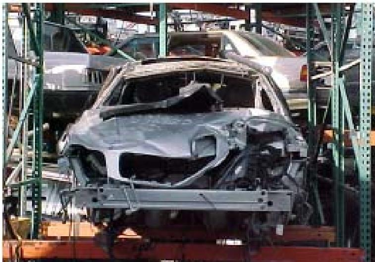
Fig. 8: 2003 Volvo XC90 showing the desirable performance during rollover. The two belted first row occupants were uninjured in the 1.5 roll collision [Hinojosa, 2003]. Roof shows very modest upward tenting of header.
