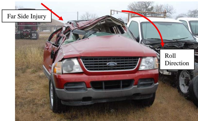
Fig. 3: Results of rollover showing disproportionate damage to initially trailing side. Note that 95% of rollovers are 2 revolutions or less [Hare, 2002].
