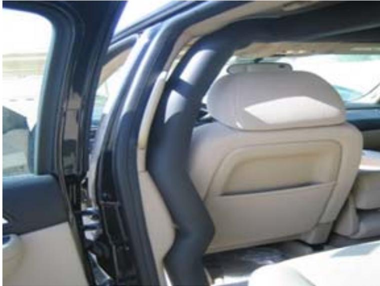
Fig. 6: Internal roll bar system designed to minimize roof crush. Notice size increase due to padding.
